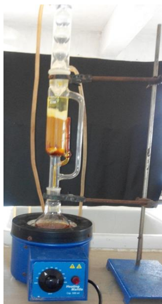
Figure 2: Soxhlet apparatus for the extraction of curcumin
