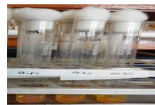
Figure 7: Immersion of acrylic strips in 0.1%, 0.2% and 0.3% of Curcumin solution for 8 h
