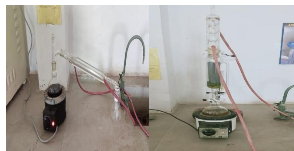
Figure 1: Soxhlet extraction and distillation of sterculia urens extract.
